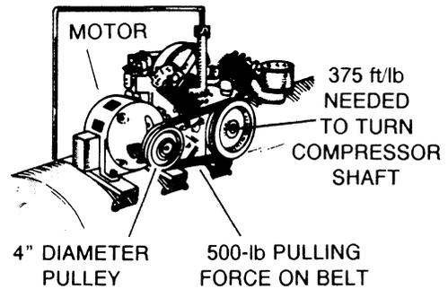
Find: The diameter of the pulley that is attached to the shaft of the air compressor. **Hint:** Remember that the diameter is 2 times the radius. The radius is the lever arm of the pulley.
