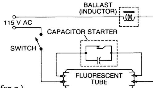
**Problem 3:** Given: In the fluorescent lamp assembly described in Problem 2 above, a ballast stores and releases the energy it takes to maintain conduction in the fluorescent tube as the AC voltage increases and decreases. The inductor rating is 3 henries at 150 milliamperes.
